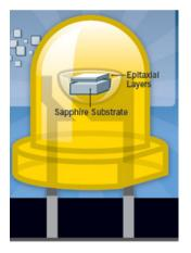
23. Rubicon sells sapphire to LED manufacturers at various stages in the process, depending on how much finishing the customer does on its own. For example, one LED manufacturer may purchase cores from Rubicon and then perform the slicing, polishing and patterning itself, whereas another LED manufacturer may purchase polished wafers.
